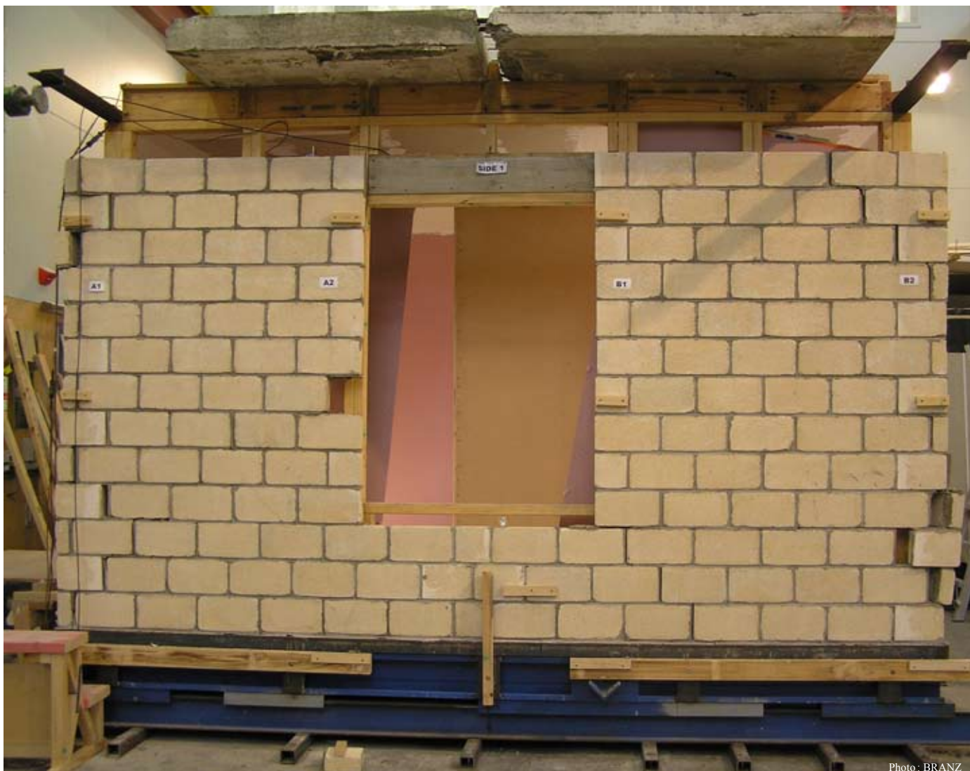
Brick veneer shake table testing.
