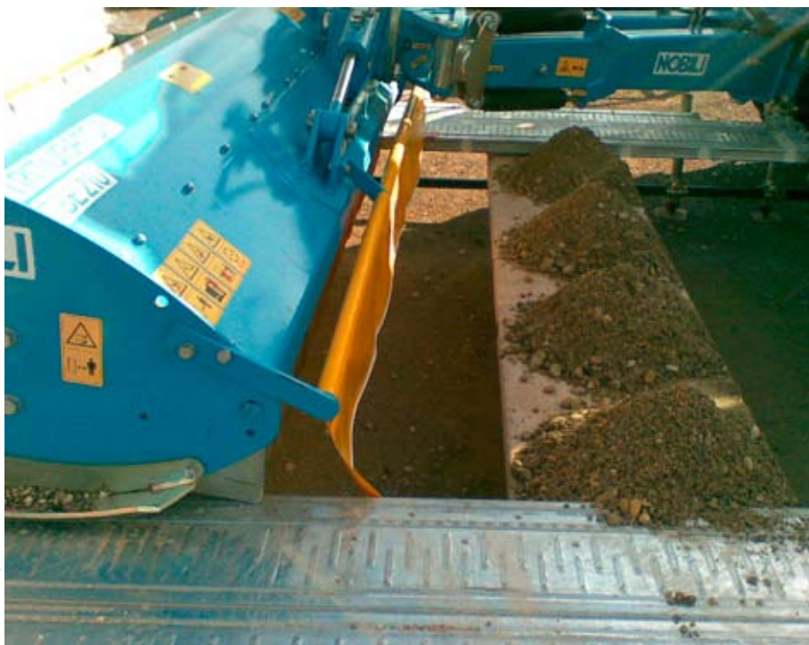
Flail mower transverse preparation testing of thrown objects over stone and gravel composites.
