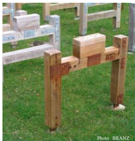
Fastener corrosion exposure site.
