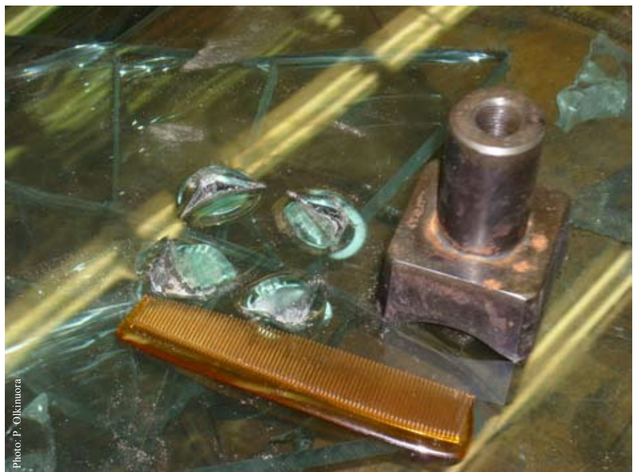
ISO 11839 specifies testing criteria for glazing and panel materials used in an operator enclosure to protect against thrown sawteeth. Pictured here, collision of a four-pointed saw tooth on a polycarbonate window.
