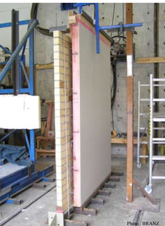
Brick veneer testing in the structures lab.
