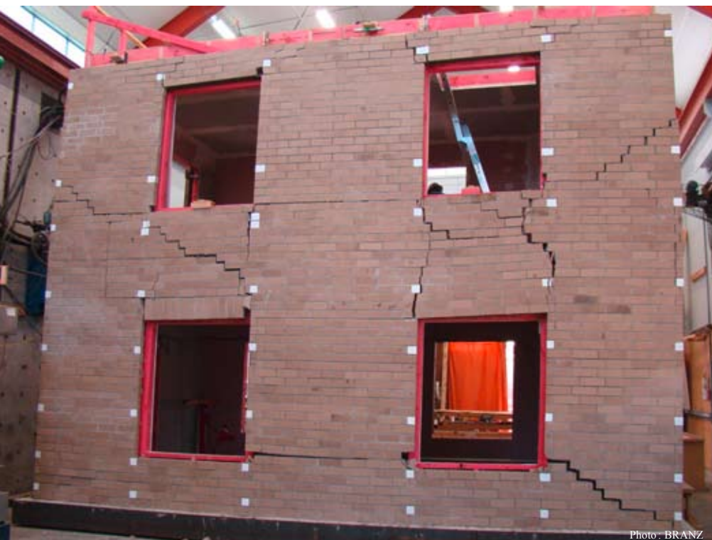
Two storied brick veneer post shake table testing.
